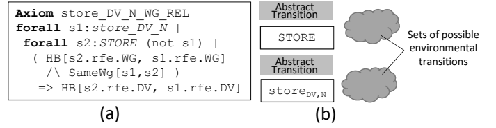
Fig. 7. (a) An axiom for instruction store_{DV,N} (b) related program sketch GPU performs a series of operations to achieve the effect of an instruction in the high-level specification. These operations are modeled as child instructions, which make use of the physical locks, FIFOs, and caches to guarantee correct data transfers and orderings.
